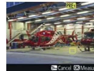
Spot White Balance setting screen (Yellow square indicates Spot White Balance target to acquire preset manual data)
