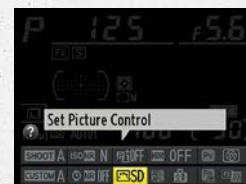
During optical viewfinder shooting: Quick change of settings is available on the information display even when the LCD monitor is turned off
